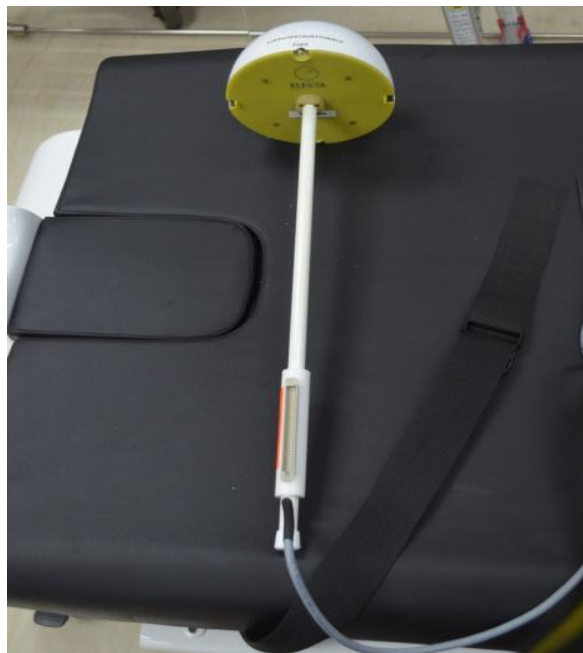
Figure 1: Reference phantom (RefPhantom) NM24058N (Serial number: 101861) provided by Elekta Oy, Helsinki Finland. 32 built in simulated dipoles and four presetting head position indicator coils (HPI).
