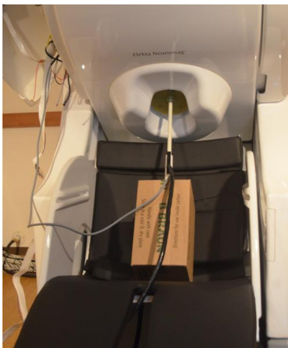
Figure 3: Phantom is carefully set into sensor helmet of the probe unit and pushed again helmet. HPI coil is fitted into outlet under right gantry side cover.
