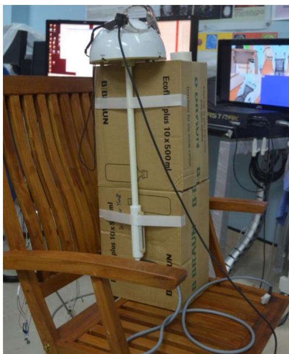
Figure 2: The digitisation of the phantom including the head positioning indicator (HPI) coil (4 point).
