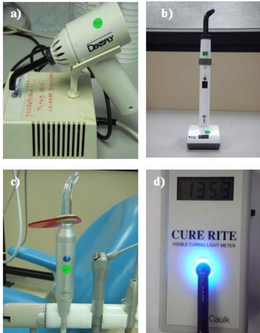
Fig. 1 a) QTH LCU. b) Cordless LED LCU. c) Cabled LED LCU. d) Measuring the light intensity output using a radiometer.
