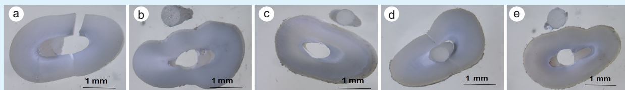
a: mixed failure; b: adhesive cohesive failure; c: adhesive-to-dental interface failure; d: dentin cohesive failure; e: fiber post-to-adhesive interface failure
