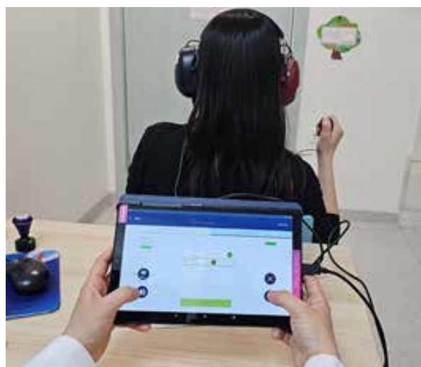
Pic 2. Hearing screening using the MAICO easyTone device at a primary health care clinic in Ulaanbaatar, Mongolia. The participant is seated with their back to the examiner and wears DD65 v2A sound-attenuating headphones. Screening was performed beginning with the right ear at frequencies of 1000, 2000, 4000, 6000, and 500 Hz in a fixed sequence, followed by the left ear. Upon perceiving the stimulus tone, the participant presses the response button. The examiner administers the screening via the tablet and continuously monitors ambient noise levels in real time.
