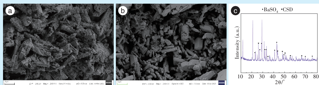
a: the SEM image of the sealer after 48 h of hydration showing needle-like crystals; scale bar = 5 \mu m; b: the SEM image of the cured sealer after dissolution for 30 d showing short rod-like crystals; scale bar = 5 \mu m; c: X-ray diffraction image of the sealer after 48 h hydration. The main components of the sealer were CSD (the hydrated CSH) and BaSO 4 . CSD: calcium sulfate dehydrate. CSH: calcium sulfate hemihydrate. Group G4: 80 wt% CSH; 20 wt% BaSO 4
