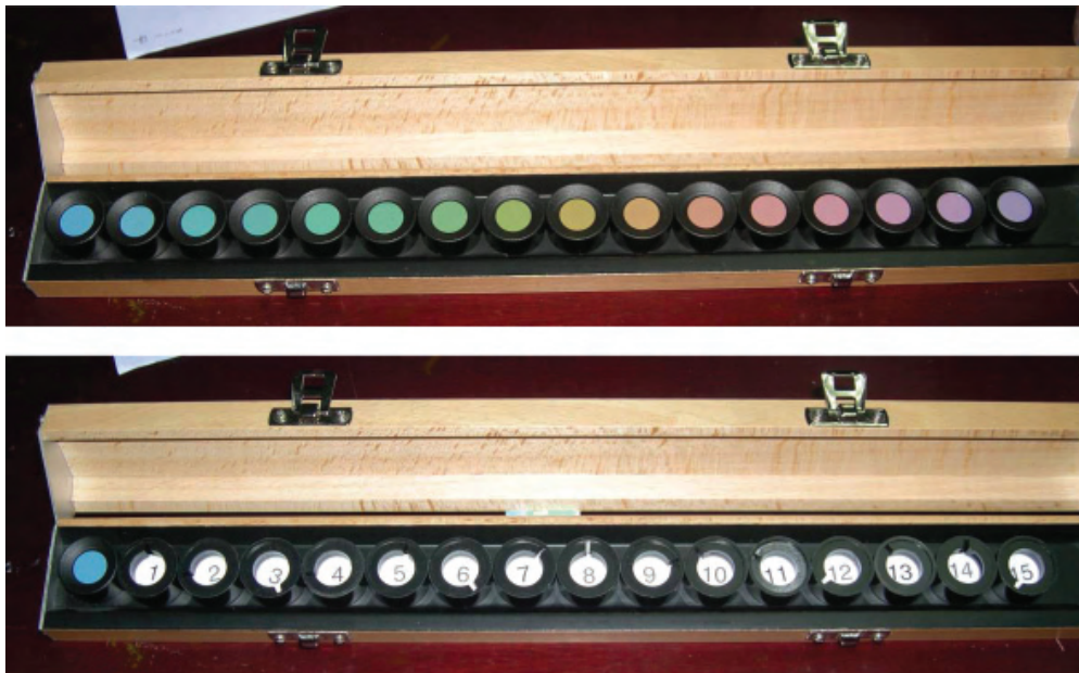
Figure 1. Farnsworth Panel D-15 hue test equipment. Different colour caps put in the black square socket; reverse side of the socket with the discs showing the serial number from 1-15.
