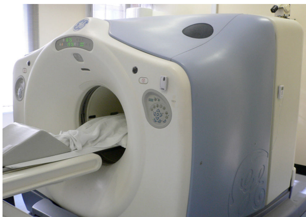
Figure 2 The Discovery LS (GE Medical Systems, Milwaukee, WI) was the first commercial PET-CT scanner to become available. This scanner at these authors' institution was installed in 2001 and has now performed over 12,000 scans. Implementation of this scanner involved end-by-end installation of a 4-slice Lightspeed plus CT with the GE Advance NXi PET scanner with a new patient bed. The CT and PET components operated on independent computer platform.
