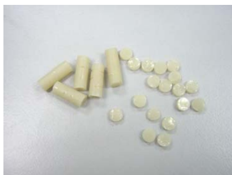
Figure 1: Composite resins after being packed in drinking straws and sectioned into discs.
