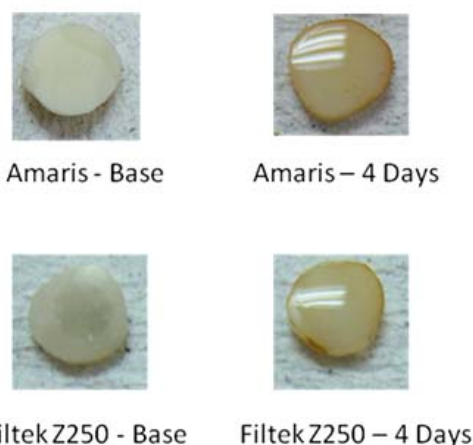
Figure 2: Comparison of the effect of staining of Filtek Z250 and Amaris at baseline (Left) and after 4 days (Right) in coffee solution.
