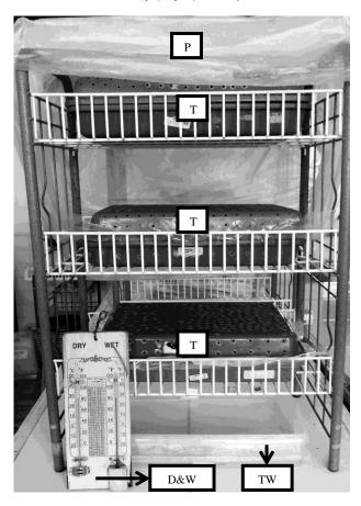
**Figure 1:** The tray fermentation system; T, perforated tray; D&W, dry and wet bulb thermometer; P, plastic covered the rack fermentation; TW, bottom tray filled with water; P and TW were used to keep the desirable humidity and temperature.
