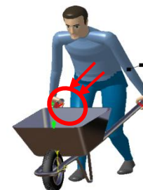
Figure 4 - shows the worker may have to bend his body in an awkward posture when pushing the heavy wheelbarrow with forced wrist and finger exertion
