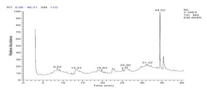
**Figure 1:** GC-MS analysis of EEST. Analysis was done with Thermo GC-Trace ultra (VER: 5.0) coupled with thermo MS DSQ II using DB 5 MS capillary standard non-polar column (diameter, 30 Mts; ID, 0.25 mm; FILM, 0.25 µm) and helium (He) as carrier gas (flow rate of 1.0 mL/min) at oven temp 70 °C raised to 260 °C at 6 °C/min. The sample injection volume is 1 µL.
