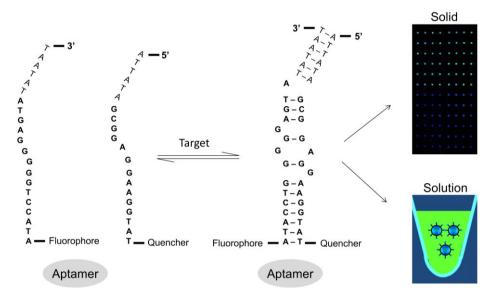
Figure 3: Bipartite aptamer. One portion aptamer carries fluorophore and another one has quencher. There will a change in the fluorescent intensity upon availability target indicates level of sensing. Aptasensor on both solid surface and in solution are shown.
