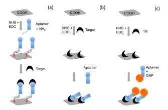
**Figure 4:** Strategies for sensing aptamer and target interaction. Strategies are shown on COOH functionalized surface. a, Aptamer (probe) vs target (protein); b, Protein (probe) vs target (aptamer); c, Signal enhancement with aptamer conjugated gold nanoparticle (GNP).
