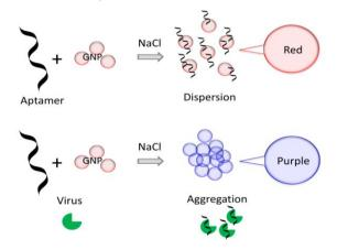
**Figure 5:** Aptamer mediated controlled assembly and disassembly on GNP. GNPs change from dispersion to aggregation in the presence NaCl, but remains dispersion in the presence aptamer. When target is available aptamer-target induces aggregation in the presence of NaCl.
