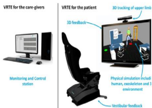
Figure 1 - The Virtual Reality Training Environments (VRTE) hardware setup for MINDWALKERS - left: care-giver training authoring and monitoring. Right: patient training environment. The upper body of this virtual human representation is controlled via the tracking data, and its legs are actuated by the Virtual Exoskeleton's controller, using BCI inputs.
