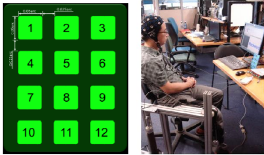
Figure 4 - Dual training protocol for SSVEP based robotic exoskeletons - left: schematics of flickering panel where 12 green flickering LEDs with different frequencies for 12 possible commands. Right: Neurorehabilitation exoskeleton setup includes the EEG cap, lower limb knee joint exoskeletons, a flickering panel and user interface.
