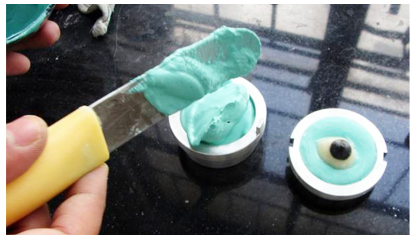
Figure 5: Investing of the wax pattern.
