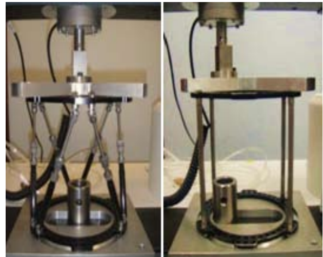
Fig. 2a: Loading test on Frame A along the midaxial line Fig. 2b: Offset axial loading on Frame C.
