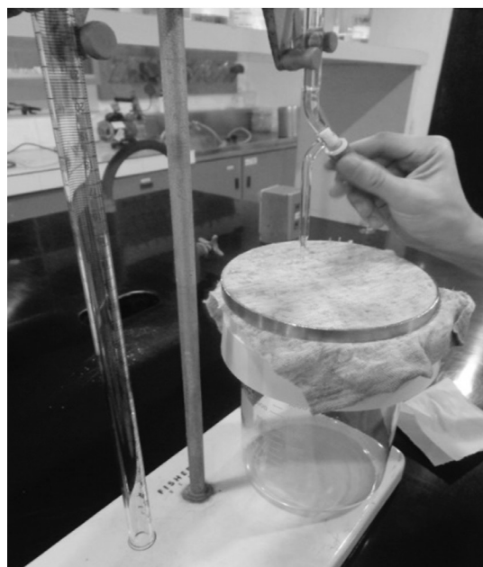
Figure 3. Absorbency test of GuaBaNIKA sock knit
