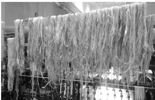
Figure 1. Banana fiber after decortication
