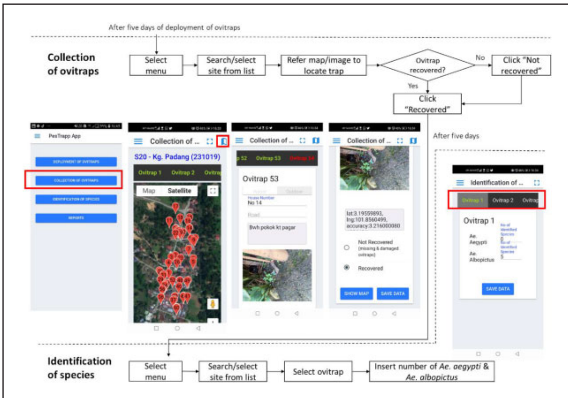
Figure 2. Screen layouts of the PesTrapp for collection of ovitrap and identification of species process.
