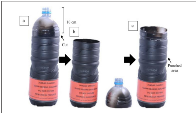
Figure 2. Construction of NPK Fertiliser Trap that was used in sampling larvae and adult mosquitoes.
