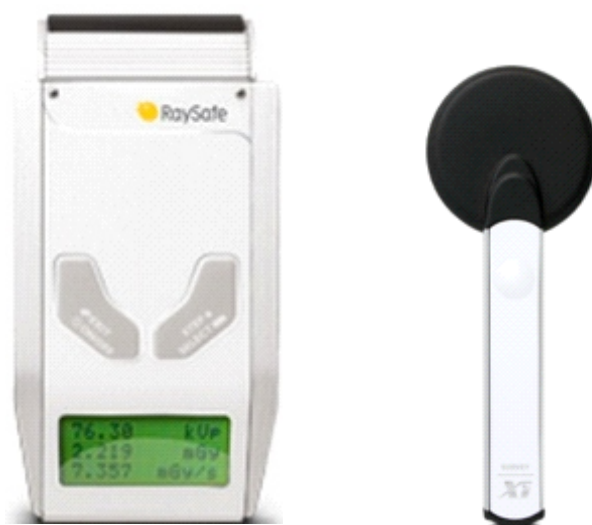
Figure 3. The survey meter that was used is the Unfors RaySafe Xi base unit and its survey measurement detector probe. (Photo Credit: RaySafe [27])
