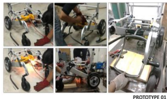
Figure 11. Assembly of lifting system on Prototype 01
