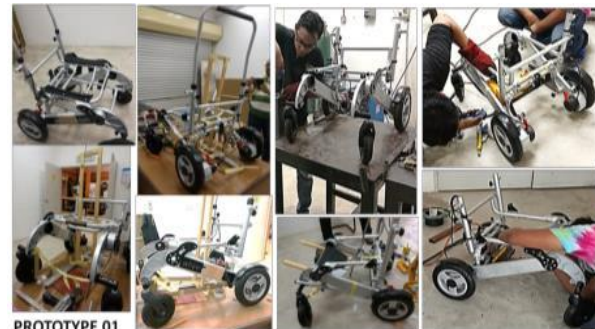
Figure 10. Reconstruct wheelchair frame
