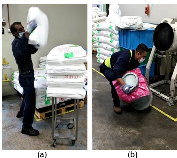
Figure 1: Manual lifting of a (a) 25-kg chemical bag and (b) 28.61-kg tumbling container
