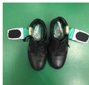
Figure 2a - F-scan sensor inserted in the safety shoes
