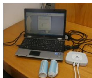
Figure 2c -F-scan software display at the laptop
