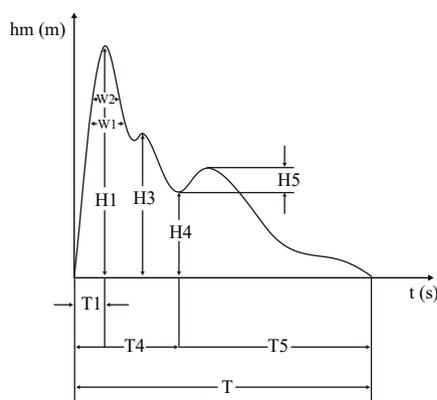
**Figure 1** One representative cycle of a pulse waveform and time domain parameters of the pulse diagram
