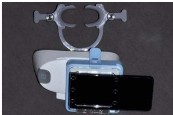
Fig. 2 Scan box and dedicated cheek retractor for remote monitoring by Dental Monitoring ® with smartphone in place.
