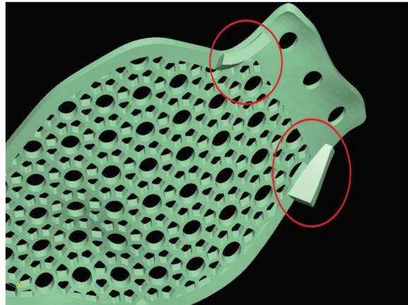
**Fig. 3** Orbital PSI design modification with placement of two implant "rest" located at the inner aspect of the inferior rim.
