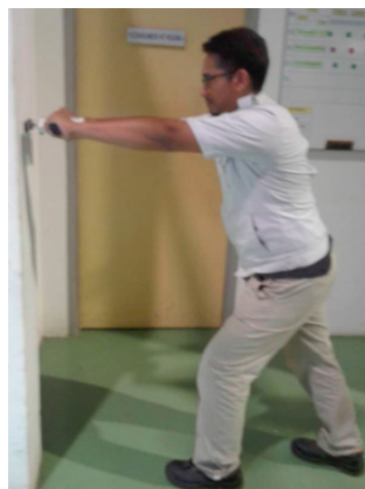
Figure 1: Action: Push; Handle height: Shoulder level; Stance: Staggered
