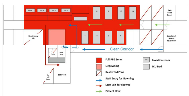
Figure 1: One-way entry-exit floor plan for restricting of ICU during the pandemic COVID-19
