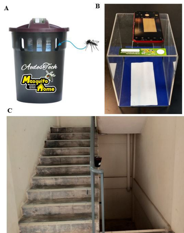
Figure 1: (A) Aedes Mosquito Home system (B) Image of eggs captured at a fixed distance before counting using 'AedesTech' Mobile App Version 5.9 (C) one AMHS fixed at each flight of stairs for Aedes mosquito egg collection.
