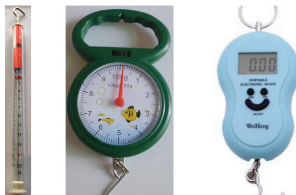
Figure 2: (a) Manual scale with accuracy 20ml; (b) Manual scale with accuracy 50ml; (c) Digital scale
