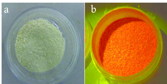
Figure 1: Nanostructured zinc oxide powder viewed under a) white light and b) ultraviolet light. Although zinc oxide powder exhibited slight photoluminescence, the intensity was not strong.
